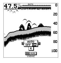
indicating the unit is in the manual mode. To turn Automatic on, repeat the above steps to get the auto menu, then press the right arrow key.
